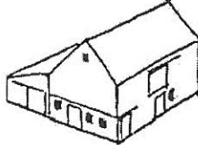
Barn with lean-to wing. Tin roof. Concrete block foundation wall in end elevation. Vertical board cladding. #14
