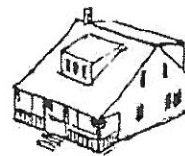
1920 #11 veranda incorporated into roof slope, shed dormers front and rear.
