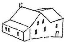
1 1/2 storey gable roof with ell 1950s
