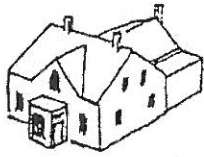
1850 #10 with flat-roofed porch and rear ell
