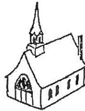
1922 #1 Quasi-Norman/ French Regime, with raked eaves and arched doorway. Stone construction.
